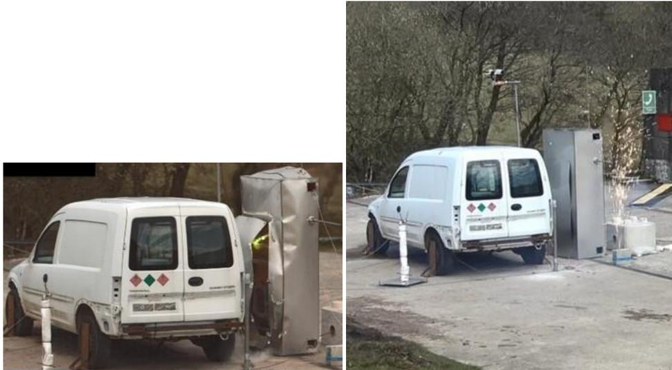
**Figure 3.1-3. Explosion of the internal flammable cloud by an internal ignition source (left TT18) and by an external ignition source (right TT20)**
