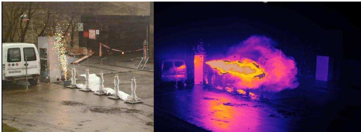
Figure 3.1-1. Standard (left) and IR image of a jet flame (right) from test TT2
