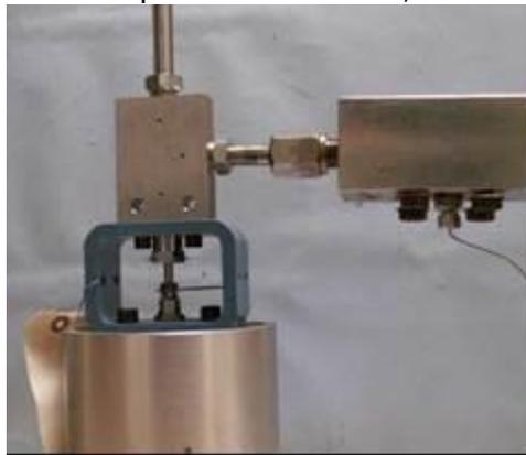
Figure 4.1-2. Air operated high pressure valve used to perform the test of figure 4.1-1
