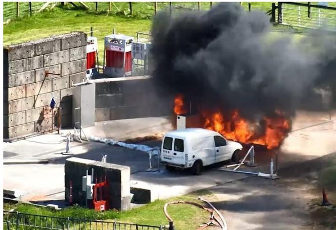
Figure 3.2-1. 120 l-2 m<sup>2</sup> diesel fuel pool fire at 2.7 m from the dispenser (TT22)
