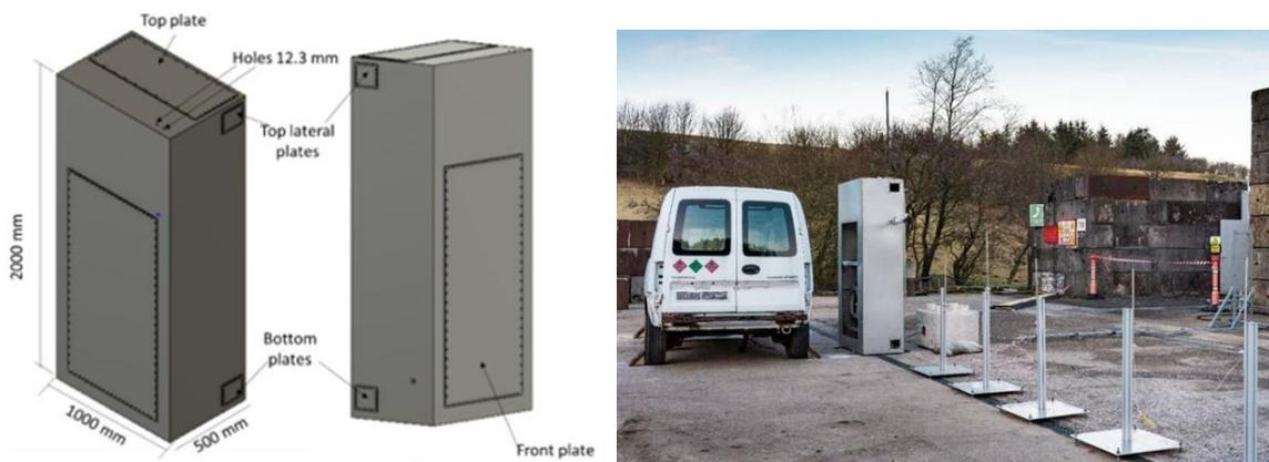
**Figure 2.4-1. Mock-up dispenser and forecourt experimental arrangement (D2.3)**
