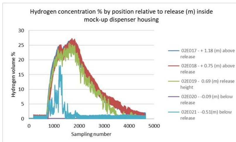
**Figure 3.1-2. concentration of H<sub>2</sub> in the dispenser on the vertical axis during test TT04 (10 sampling points for 1 s)**
