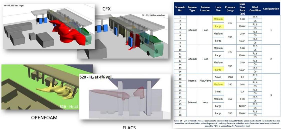
Figure 2.2-4. Location of the Lower Flammable Limit isosurfaces for typical release scenarios (D2.3)
