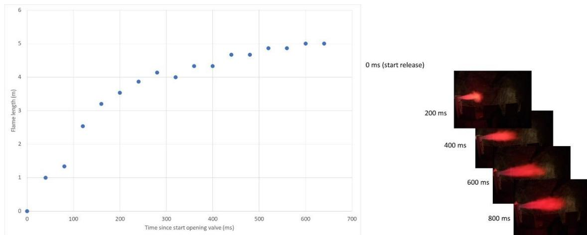
**Figure 4.1-1. evolution of the flame length in a horizontal flame jet issued from a 2 mm orifice under 900 bar (80 g/s)**
