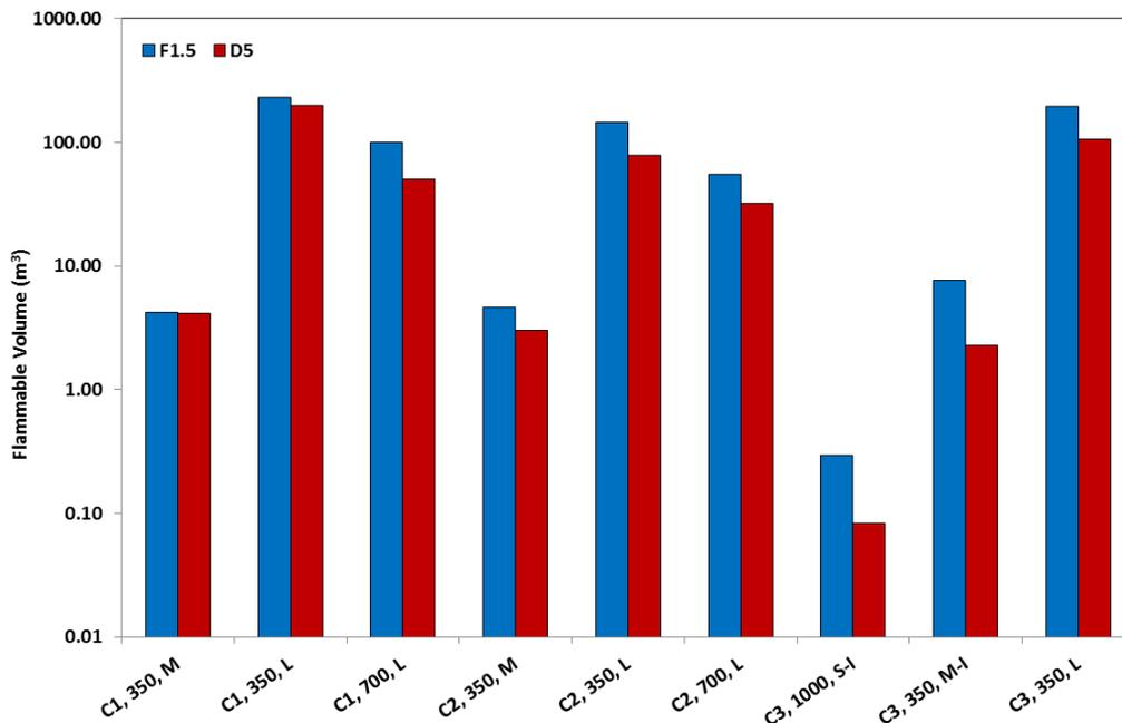
Figure 2.2-5. Volume of the flammable zone as function of the scenario and atmospheric conditions (D2.3)
