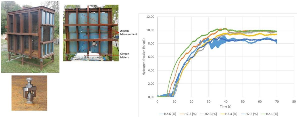
**Figure 4.2-1. experimental configuration from Duclos *et al.*, 2017. 4 m<sup>3</sup>, upwards H2 release of 3.81 g/s**
