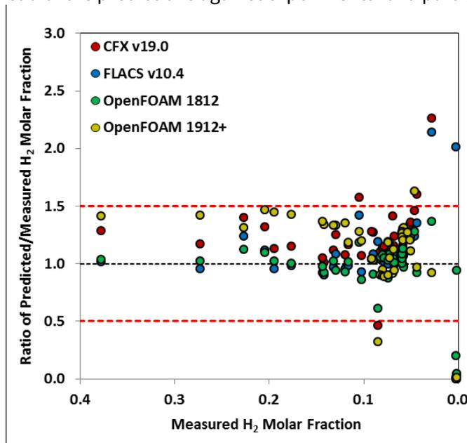
**Figure 2.2-3. Ratio of predicted-to-measured concentration (from D2.3) as a function of H<sub>2</sub> molar concentration for the unobstructed free jet scenario. Figure includes both centreline and radial data**
