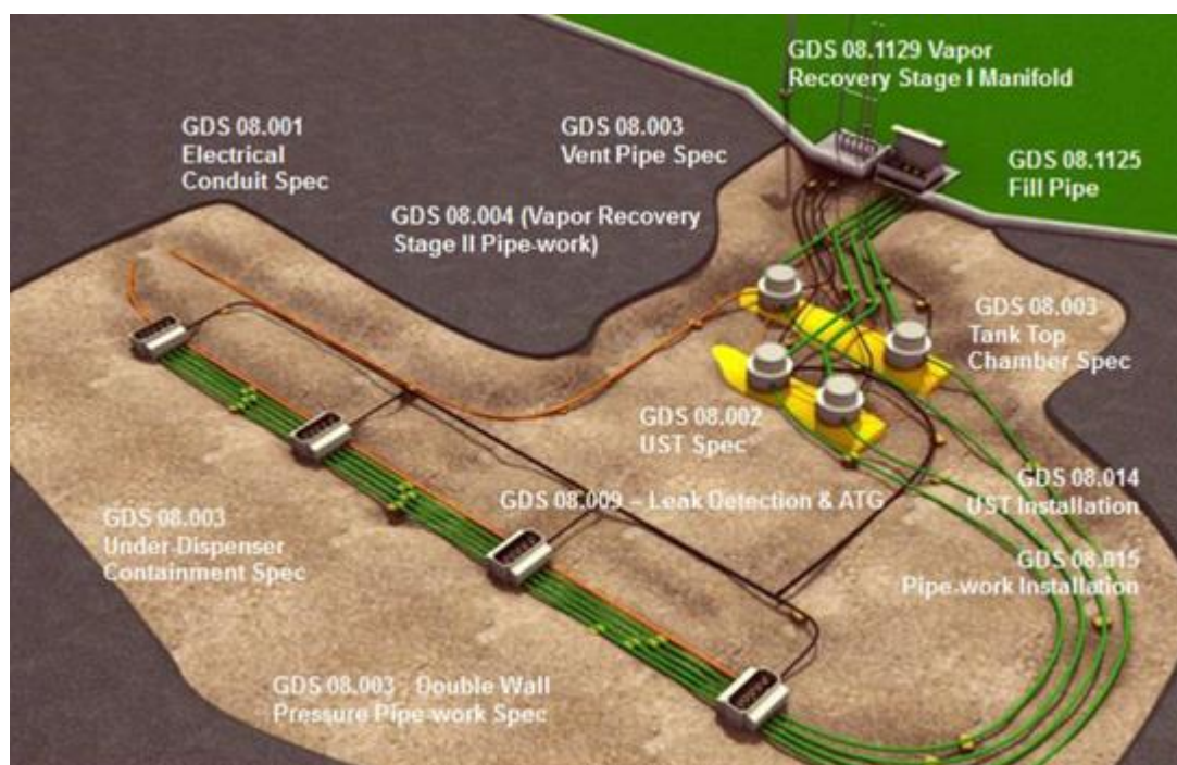
Figure 40 - Schematic of a general underground fuelling system layout including relevant Global Design Standards (GDS) per equipment item.
